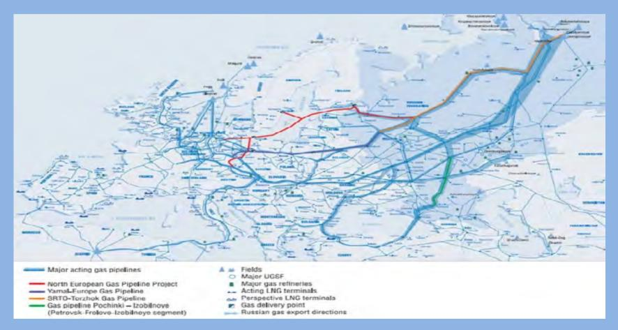
UGSS includes 155 000 km gas mains and branch pipelines, 268 compressor stations and gas-pumping units with a total power of 44.8 mln kW of gas pumping units, 6 gas processing and gas condensate complexes, 24 UGS facilities. 7
