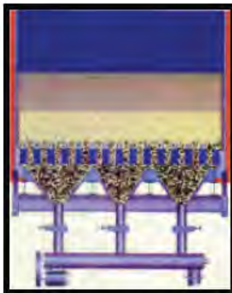
Hydro beam grate: 8,1 x 8 m, 65 m 2 , 170 MW
